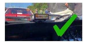
This is how the device is fitted correctly. Centre of the dash with the front of the device facing Driver and Co-Driver, able to see the red flag and function buttons. The antenna is within view of the windscreen giving optimum connection.
