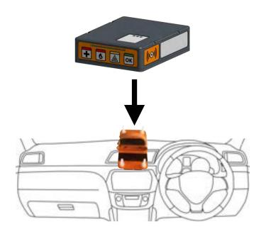
The device must be fitted in the centre of the dashboard accessible to both Driver and Co-Driver.
